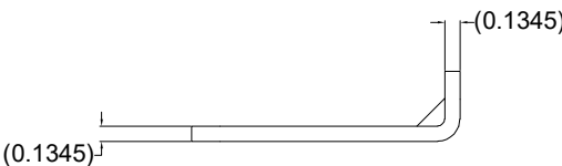
⑨ WINDLOCK DETAIL, CP1514 STAMPED STEEL IN ACCORDANCE WITH ASTM A36 OR EQUIVALENT, GALVANIZED IN ACCORDANCE WITH ASTM A123, GRADE 85 ZINC-COATING 1/2 SCALE
